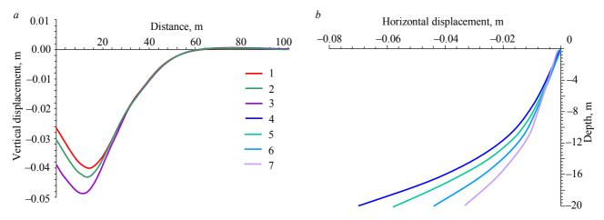
Fig.4. Graphs of vertical (a) displacements of surface in clay N 1 with different depths of «slurry trench» (model 1) and diagrams of horizontal displacement of «slurry trench» (b) with different clays (models 1-4)
