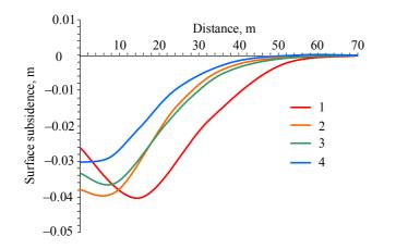
Fig.6. Graphs of vertical displacement of surface (depth of slurry trench is 800 mm) in clay N 1 for 2D (1) and 3D models with different excavation length (2-4 – 35; 30 and 40 m respectively)
