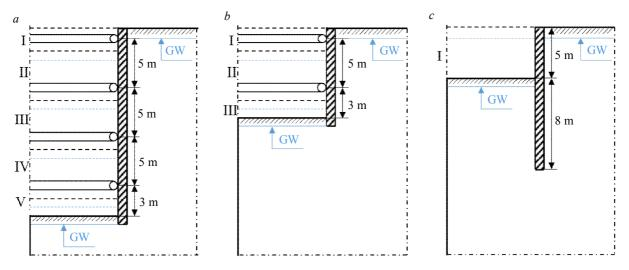
Fig.3. Excavation models: a-c – the depth of an excavation is 19, 9 and 5 m respectively; the cantilever pattern I-V – excavation stages
