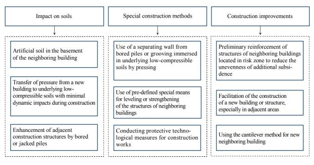
Fig.2. Classification of measures aimed at reducing the negative impacts from construction on neighboring buildings
