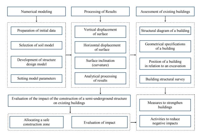
Fig.1. Algorithm for calculating semi-underground structures
