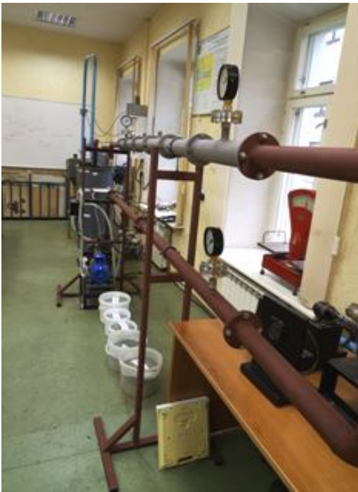
Fig.1. Laboratory hydraulic transport installation
