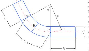
Fig.1. The offset of the first type according to GOST 24950-81  $\alpha$  – bending angle;  $D_{o}$  – offset outer diameter;  $\rho$  – offset curvature radius;  $l_1$ ,  $l_3$  – length of straight ends of the offset,  $l_2$  – length of elbow part
